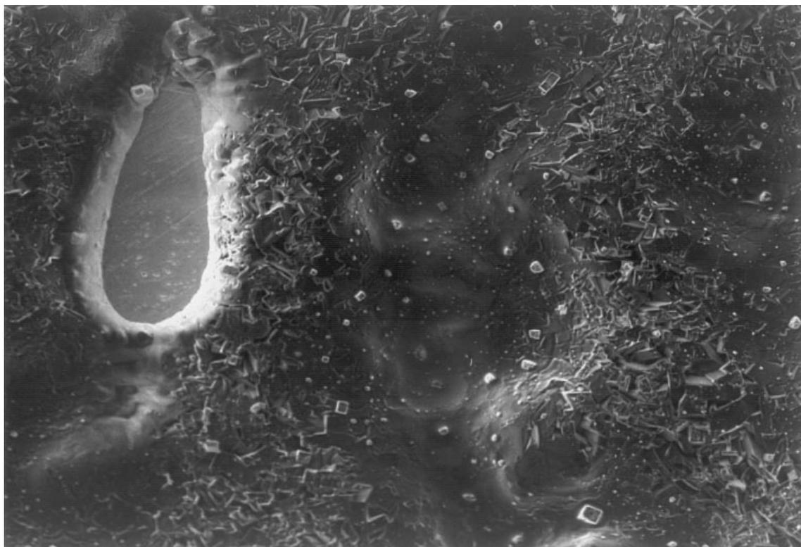
**Figure 1.** Scanning electron microscope image of a PEG 2000 sample. The image shows microfine particles produced by the aerospray technique. Laser spot size,  $80 \times 210 \mu\text{m}$ .
