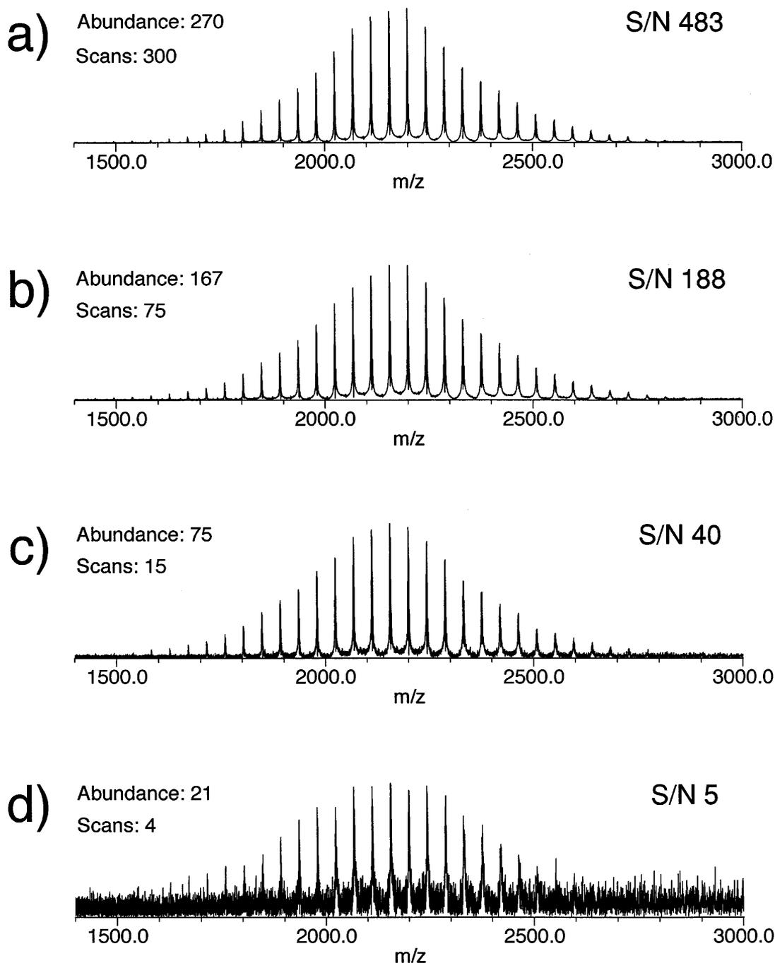
**Figure 2.** Example spectra of  $5.1 \times 10^{-7}$ ,  $5.1 \times 10^{-8}$ ,  $5.1 \times 10^{-9}$  and  $5.1 \times 10^{-10}$  mol of PEG 2000 loaded on to the probe tip. The material present on the probe allowed for signal averaging in the following amounts: (a) 400, (b) 100, (c) 20 and (d) 4 shots.
