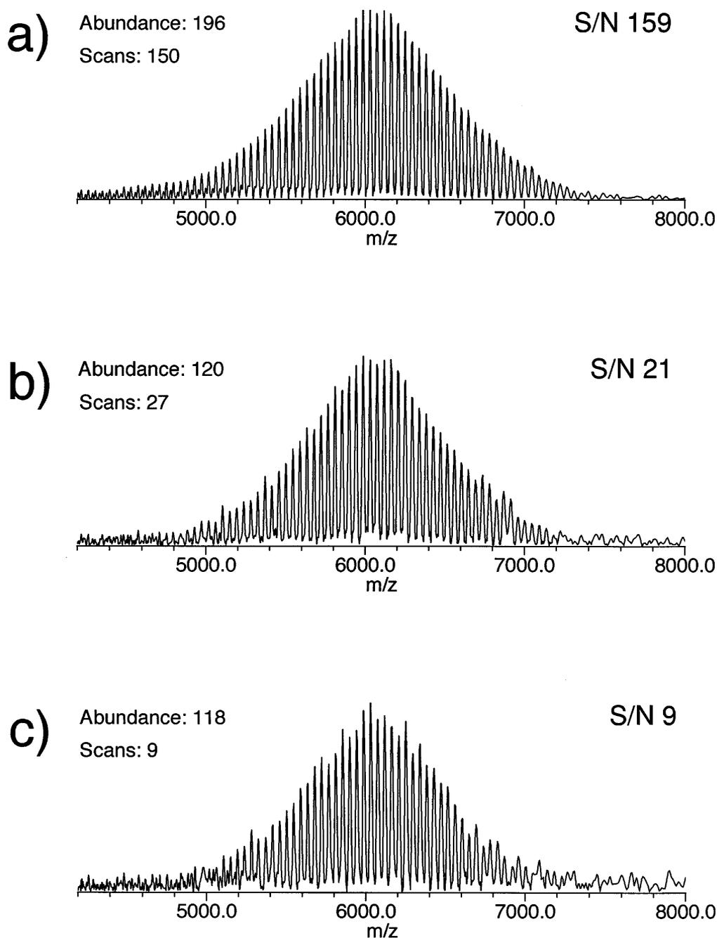
**Figure 4.** Example spectra of  $3.6 \times 10^{-7}$ ,  $3.6 \times 10^{-8}$  and  $3.6 \times 10^{-9}$  mol of PEG 6000 loaded on to the probe tip. The material present on the probe allowed for signal averaging in the following amounts: (a) 200, (b) 36 and (c) 9 shots.
