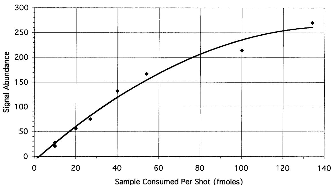
Figure 3. Plot of signal intensity vs. sample consumed per shot (in femtomoles) for PEG 2000.
